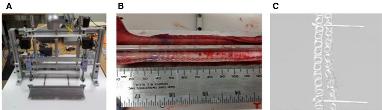
**Fig. 2** **A** Standard Bariatrics Tissue Measuring Device used to measure gastric tissue thickness. **B** Experimental staple line pictured adjacent to the ruler on the “sliver” of tissue sent for CT scanning. The
