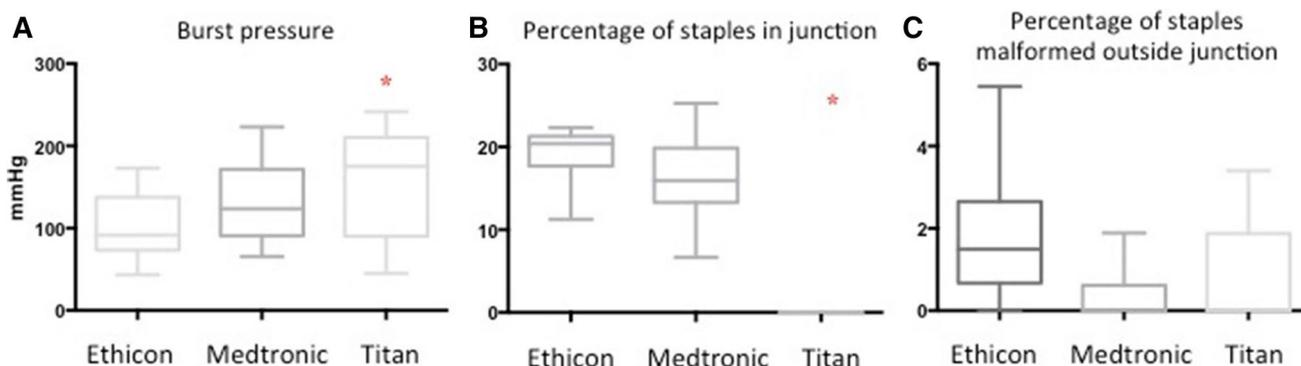
**Fig. 3** **A** The gastric remnants created using a Titan stapler withstood a significantly higher average burst pressure at 159.8 mmHg than Ethicon (102.1 mmHg) and Medtronic (128.0 mmHg) linear cutting staplers ( $p=0.01$ ). **B** Medtronic and Ethicon staplers had a similar percentage of staples measured within junctions of the speci-
