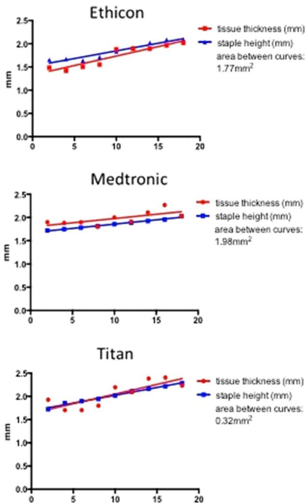
**Fig. 4** A linear regression was performed using the average staple height and tissue thickness from each stapler type, and the area between the curves was determined. Titan stapler had the smallest average difference between the two curves
